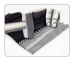
Bend down the seam while ensuring that the cloth remains fastened.
