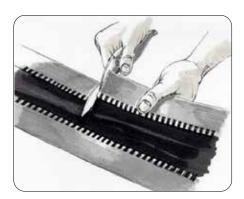
At a notch, cut a length equivalent to the perimeter required plus an overlap of 100 mm.
