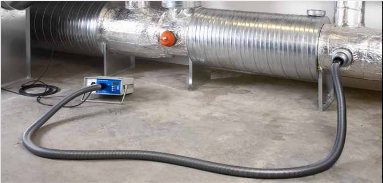
Figure 3: Connection to the duct system
